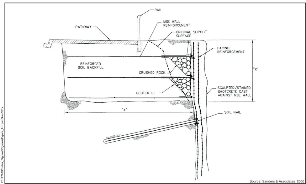
Under Alternatives 1 and 2, mechanically stabilized earth would be used to help support buildout areas for parkway development.
